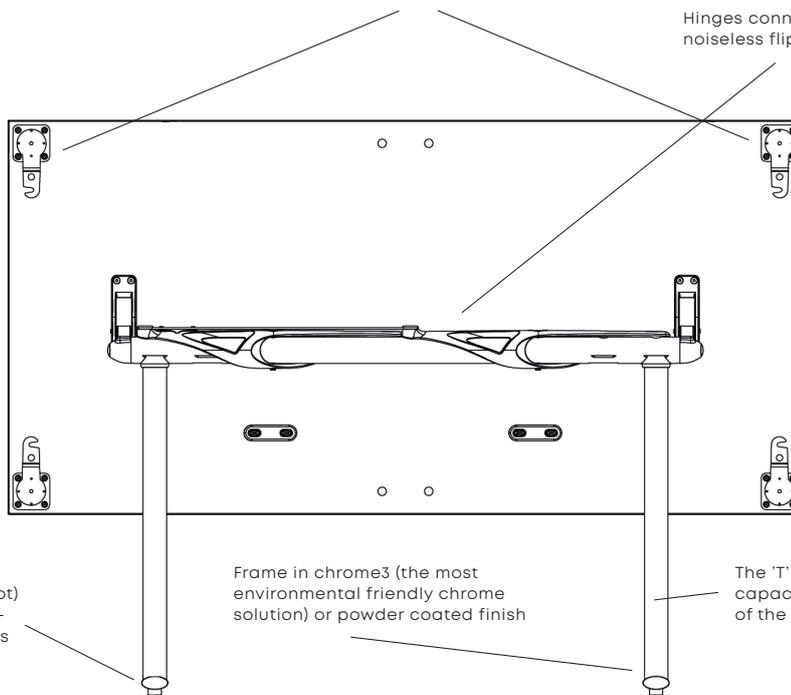
The Tempest table is considered the world's leading flip-top table system in terms of its unique space-saving and manageability qualities. Tempest is often referred to as the "zero weight" table system by combining a flip-top mechanism and integrated castors allowing the table to be moved around easily. When not in use, the tables can be nested to optimise space.
