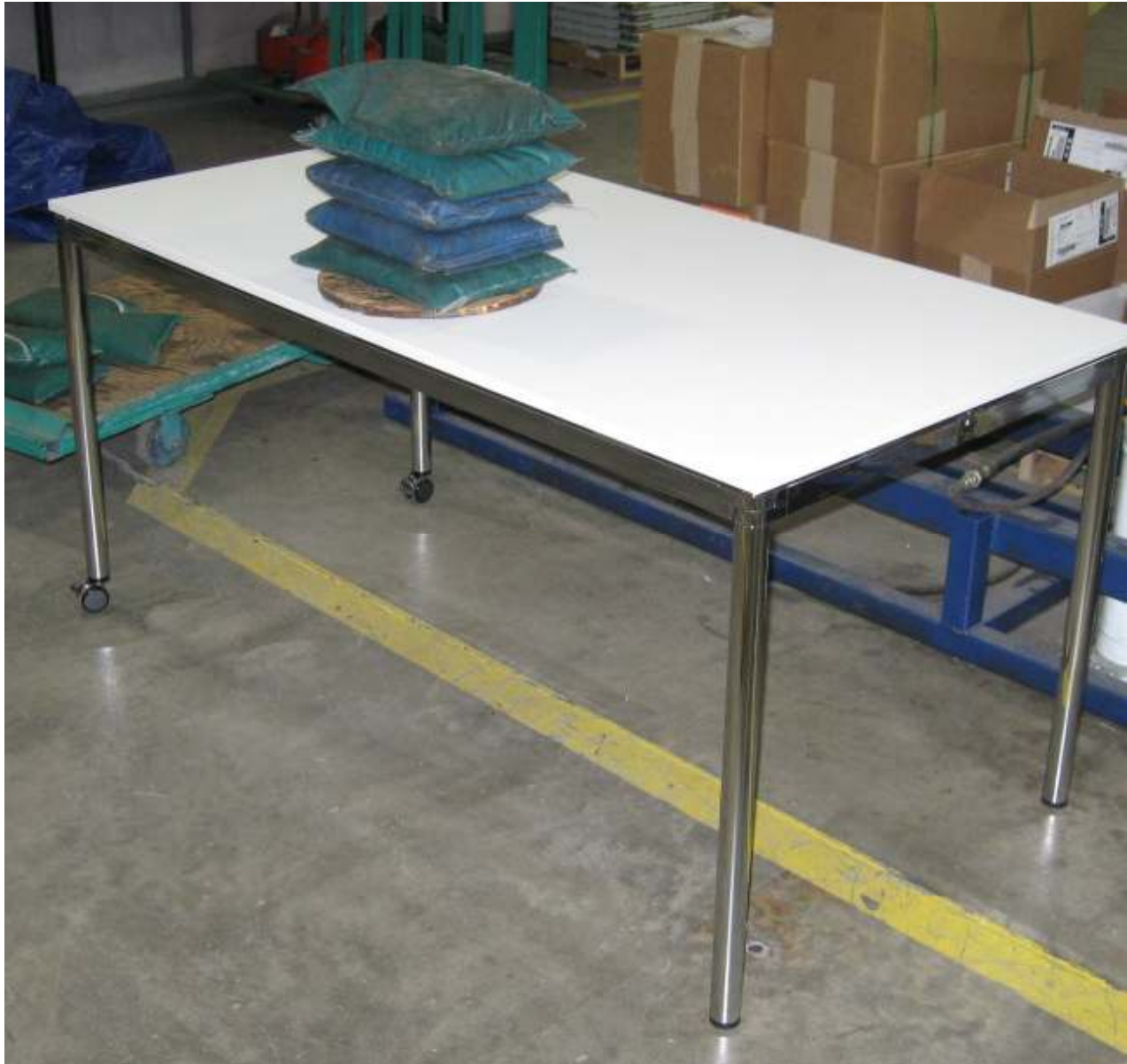
Stability Under Vertical Load Test
