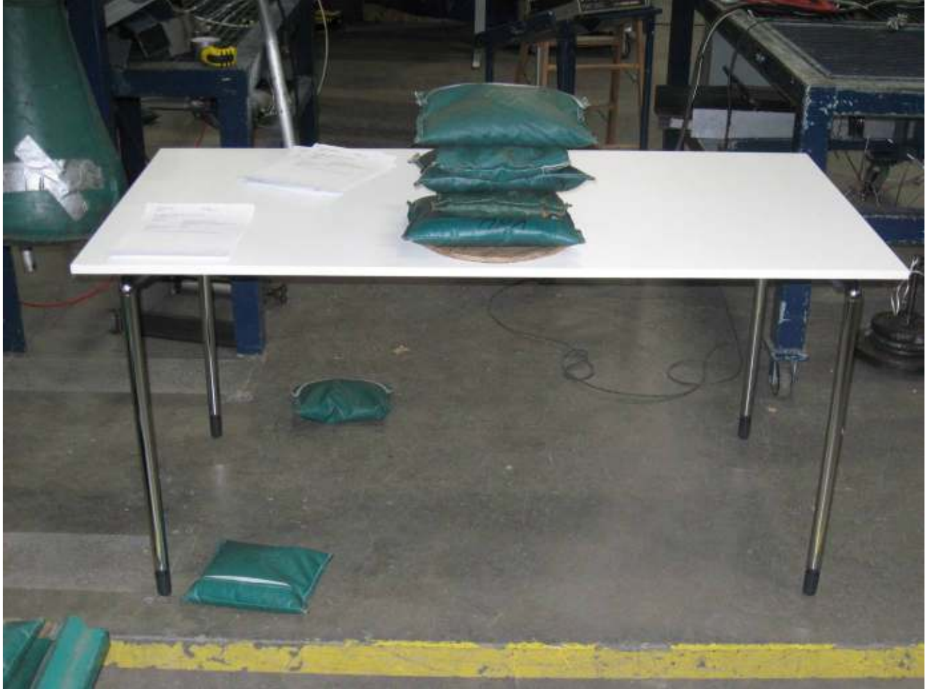
Stability Under Vertical Load Test
